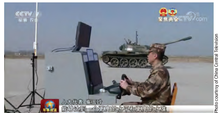
Video footage showing a Type 59 medium tank with a PLA soldier possibly controlling via a remote computer terminal.
